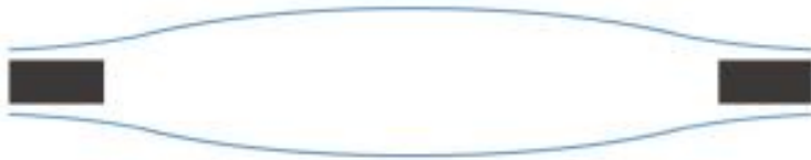
3) Concave (center is thicker than particle's minor axis)
